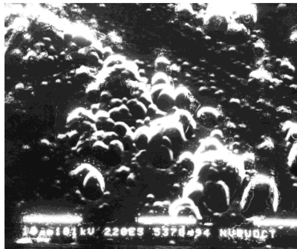
Figure 10 Electron micrograph of film deposited on glass plate for 45 min.
